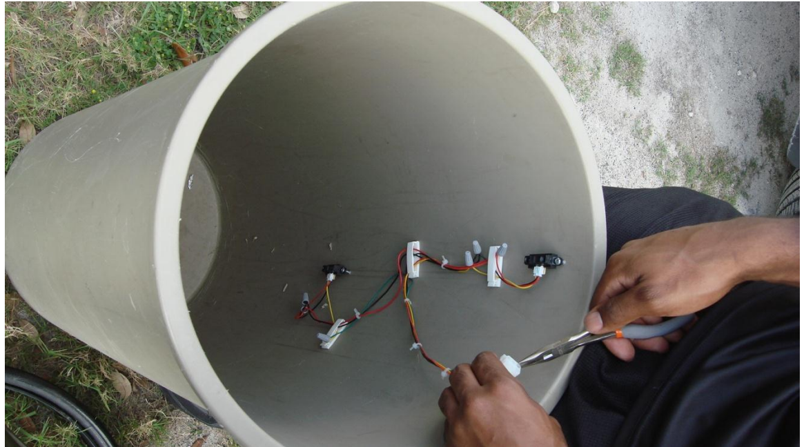
Figure 14: Can liner and sensor Mounting
